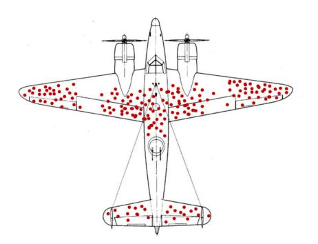
During World War II, researchers from the Center for Naval Analyses had conducted a study of the damage done to aircraft that had returned from missions, and had recommended that armor be added to the areas that showed the most damage.
